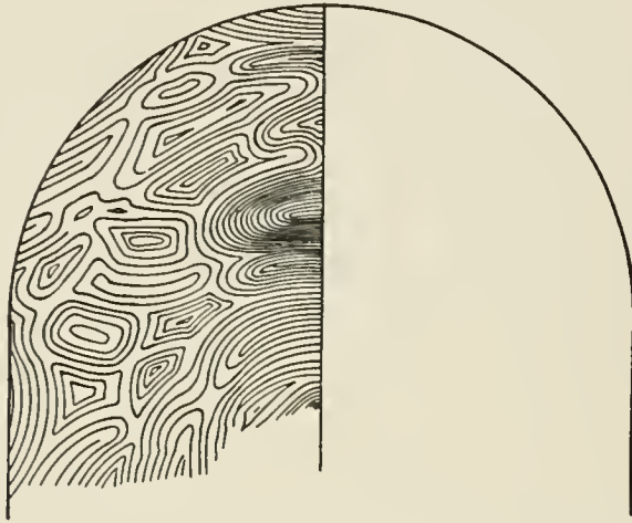
FIG. 5. Interference system for tenor C in the Kuppel-Horizont, having a thirty-six foot proscenium opening. The intensity of sound is represented by contour lines, the maximum variation being forty-seven fold.
