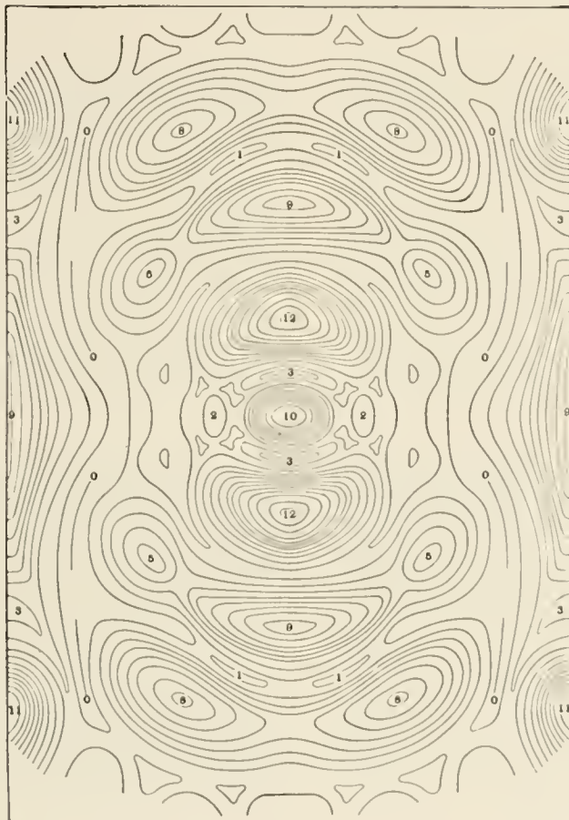
FIG. 8. Distribution of intensity on the head level in a room with a barrel-shaped ceiling, with center of curvature on the floor level.
