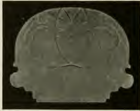
FIG. 28. A photograph, one of many taken, showing in vertical section one stage of the reflection b , Fig. 21. These reflections were eliminated by the architects in the summer following the opening of the theatre, but have been in part restored by subsequent changes.
